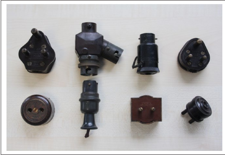
Figure 3. Pre-standardisation UK plugs and sockets. Notice the bayonet fitting light-socket adaptor (second from left). Such fittings were commonplace before the introduction of standard wall-mounted fittings. © Photograph: Damon Taylor.
